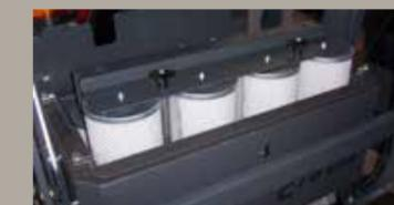
*The wide filter surface can range from 5.5 square mts in bag filters in different types of punched fabric to 6.4 square mts in cartridge polyester filters (nr. 8 filters). Depending on needs or on preferences GEMMA offers the opportunity to choose from two filter configurations. It is the action of the filter shaker that keeps cleaned the filter in both configurations.*
